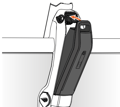
Figure 13 - Click the battery into the upper battery holder.
