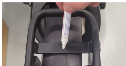
Figure 7 - Marking the drilling hole on the mudguard.
