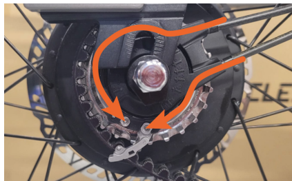
Figure 11 - Reposition gear cables.
