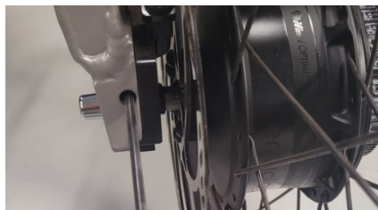
Figure 12 - Tensioning the belt.
