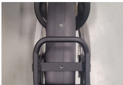
Figure 8 - Drill hole in mudguard.
