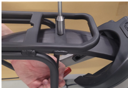
Figure 9 - Securing luggage carrier to fender.
