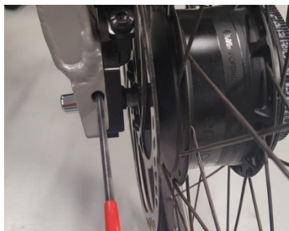
Figure 3 - Remove tension from the belt.
