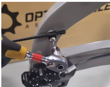
Figure 5 - Removing the mudguard rods.
