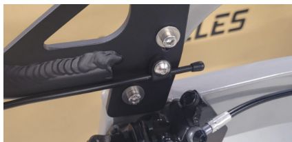
Figure 10 - Tighten luggage carrier and mudguard rods bolts.
