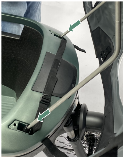
Figure 8 - Putting in the tent poles.
