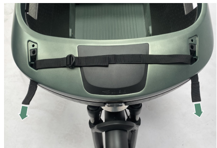
Figure 7 - Placing the mounting strip.
