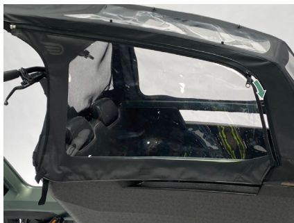
Figure 12 - Installation des portes.
