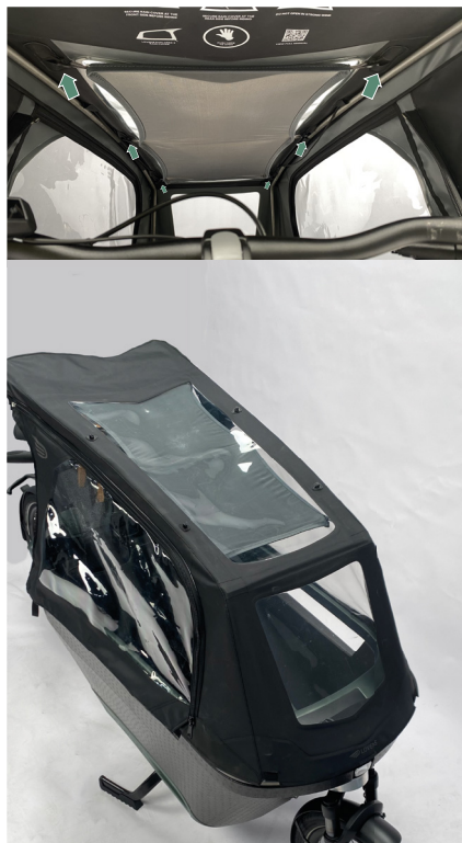
Figure 22 - Installation d'un pare-soleil.
