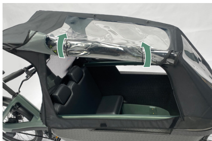
Figure 20 - Rolling up the window.
