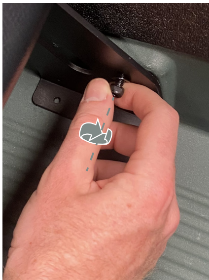
Figure 7 - Tightening bolts by hand.
