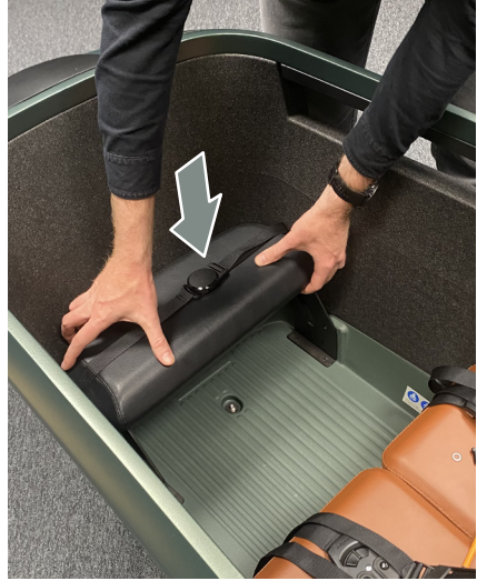
Figure 5 - Placing the front bench in the box.
