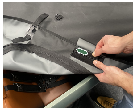
Figure 10 - Adjusting hook tension
