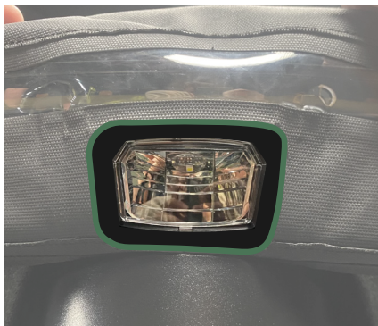
Figure 4 - Aligning the front light with the hole
