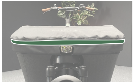
Figure 3 - Aligning the LED strip box cover
