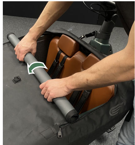
Figure 12 - Rolling up the passenger compartment
