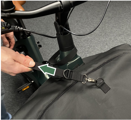
Figure 8 - Tensioning the tensioning strap
