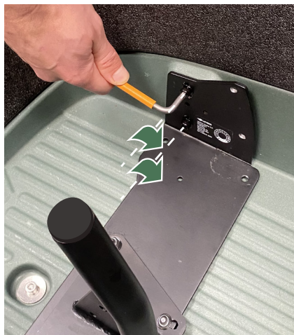
Figure 8 - Serrer les boulons.
