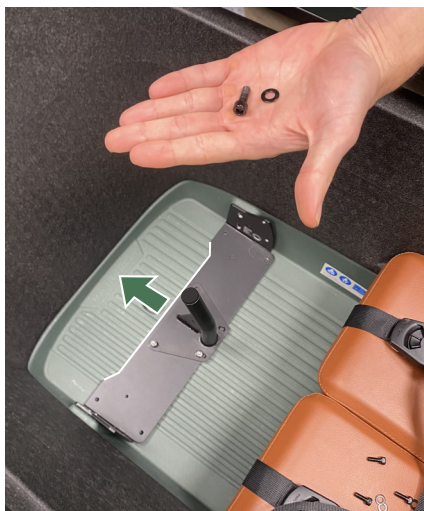
Figure 5 - Placing the child seat adapter in the box.
