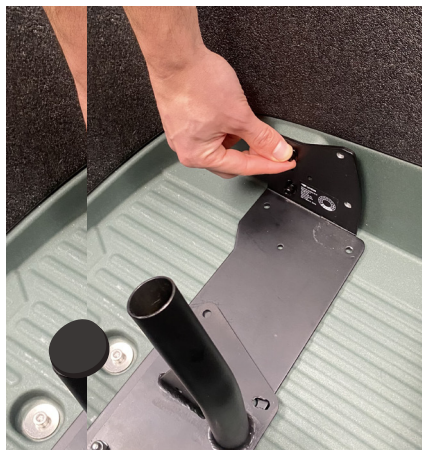
Figure 6 - Tightening bolts by hand.
