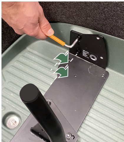
Figure 8 - Tighten the bolts.
