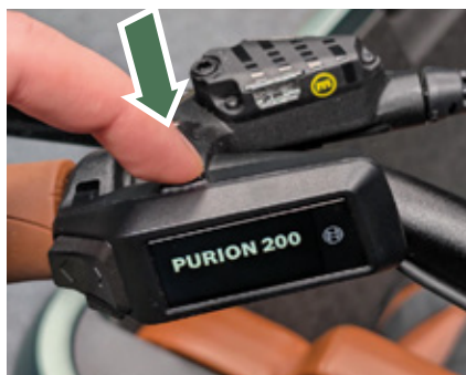
Figure 19 - Switching on the bicycle.
