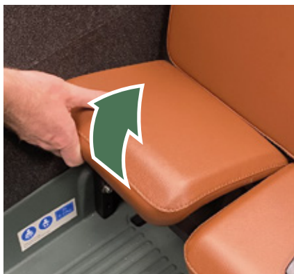
Figure 3 – Removing the seat.
