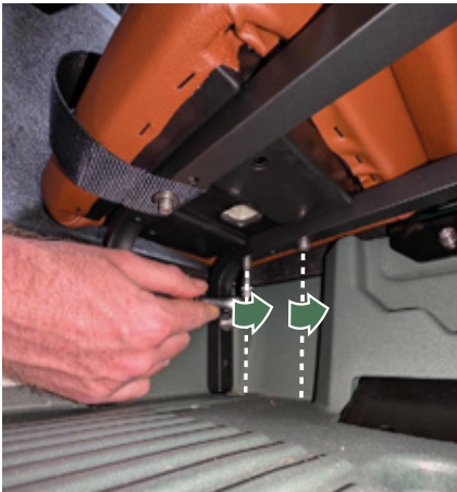
Figure 15 - Securing the rear of the heated seat.
