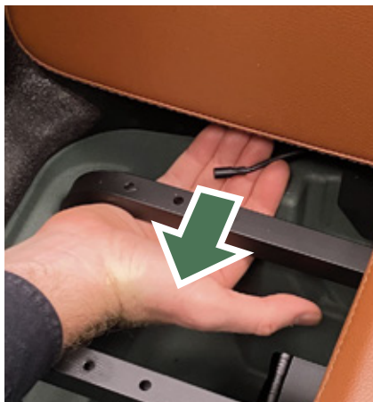
Figure 5 – Release the cable.
