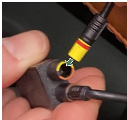
Figure 8 – Connect the yellow cable.
