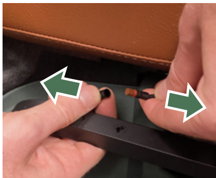
Figure 6 – Remove the cable protective cover.
