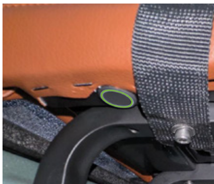
Figure 21 – Green indicator light for heated seat.
