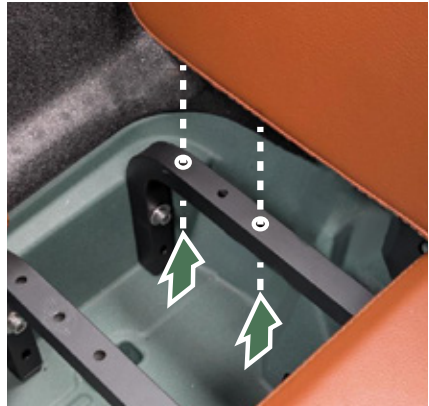
Figure 16 - Mounting holes rear.
