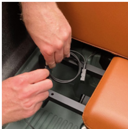
Figure 9 – Rolling up the cable.
