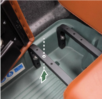
Figure 14 - Front mounting hole.
