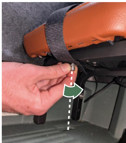
Figure 13 – Fitting the lower belt section.
