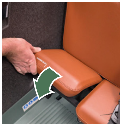
Figure 12 – Fitting the seat onto the bench frame.
